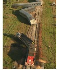
While nearing the public crossing at Secondary Highway 751, the driver of a loaded logging truck did not notice an approaching VIA Rail Canada Inc. (VIA) train. Though he swerved at the last minute, the truck collided with the north side of the lead locomotive, derailing all nine passenger cars and both locomotives. The driver of the truck sustained serious injuries and was transported to hospital. In addition, one train passenger and one VIA employee sustained minor injuries.
